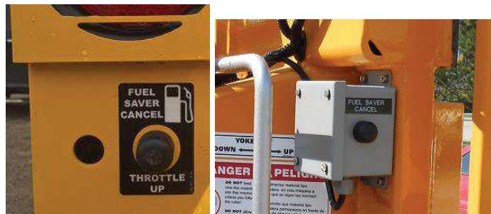
When you turn Fuel Saver OFF, the machine will throttle down to idle (approx 800rpm), EXCEPT if engine RPM is above AutoFeed Hi setting. In this case, the controller assumes the operator is at full engine speed and wants to keep working.
