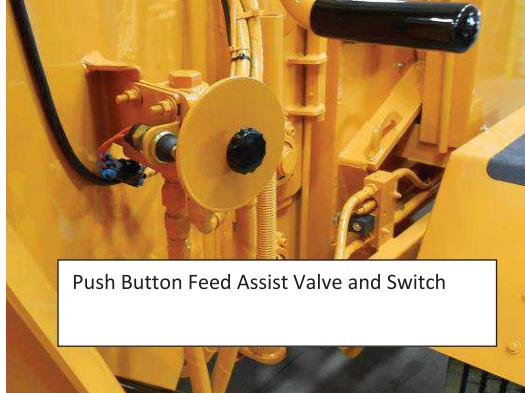
Push Button Feed Assist Valve and Switch
