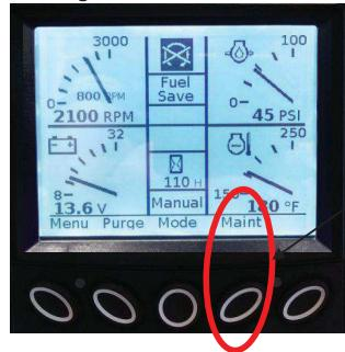
Press the Maint button to navigate to the Maintenance Pages.
