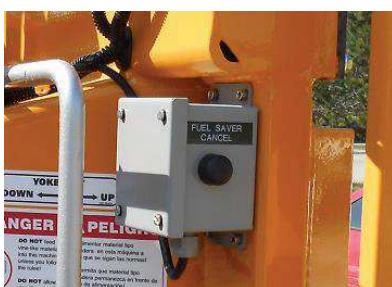
When you turn Fuel Saver OFF, the machine will throttle down to idle (approx 800rpm), EXCEPT if engine RPM is above AutoFeed Hi setting. In this case, the controller assumes the operator is at full engine speed and wants to keep working.
