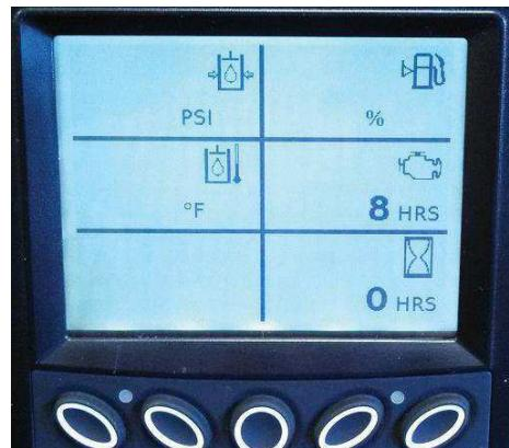
The engine may send information on other parameters it is monitoring. These can be read on 1 of 4 engine pages. Cycle through the engine pages to return to the Main Page.
