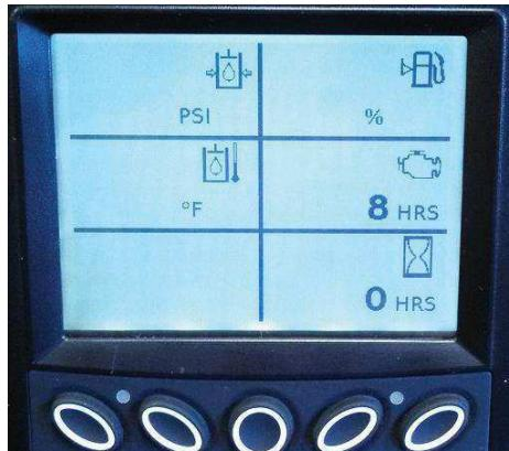
The engine may send information on other parameters it is monitoring. These can be read on 1 of 4 engine pages. Cycle through the engine pages to return to the Main Page.
