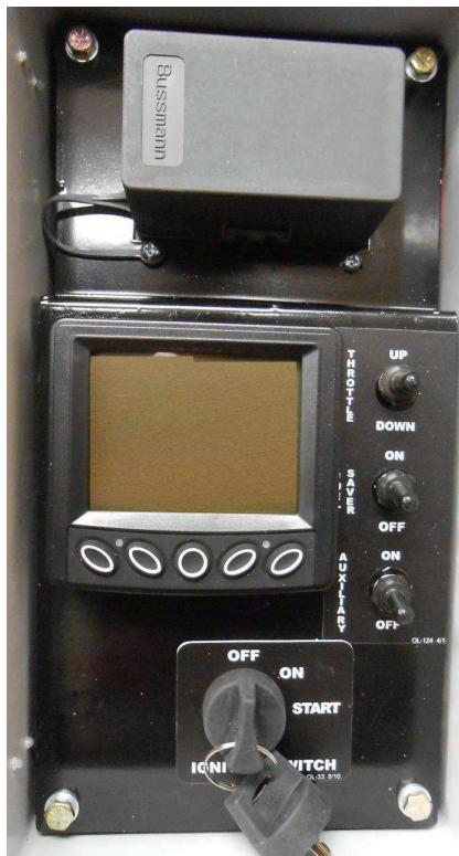
Tap Throttle Up to bring the RPM back to full speed.
