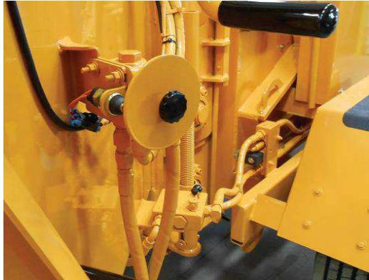
If the Chipper is equipped with a Bump Bar and Bump Bar Bypass valve, a Bypass Button is connected to the valve which together allow Feed Fwd for 5 seconds even if the Bump Bar has disabled the feed system.
