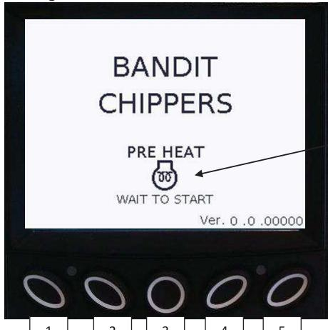
To Start, turn key to ON position. In cold weather the engine may pre heat glow plugs or heater grid and the WAIT TO START symbol will appear on the splash screen. When pre heat is complete the Display will continue to Main Page.
